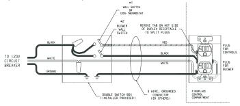
DUAL SWITCH ELECTRICAL WIRING TO FIREPLACE RECEPTACLE
